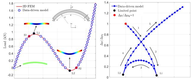
• Two methods for solving a linearized perturbed system in structural stability theory
