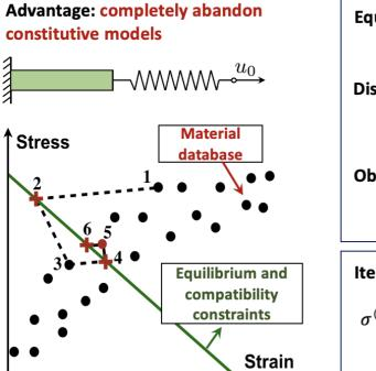
Equilibrium constraint:  $R = \sigma A - k(u_0 - \varepsilon L) = 0$ Distance penalty function:  $F = \frac{(\sigma - \sigma^*)^2}{2\alpha} + \frac{\alpha(\varepsilon - \varepsilon^*)^2}{2}$ Objective functional:  $\delta(F - \lambda R) = 0$ Iteration formulas:  $\sigma^{(i+1)} - \sigma^{*(i)} = \frac{\alpha^2 A}{kL} \left(\varepsilon^{(i+1)} - \varepsilon^{*(i)}\right)$  Results
