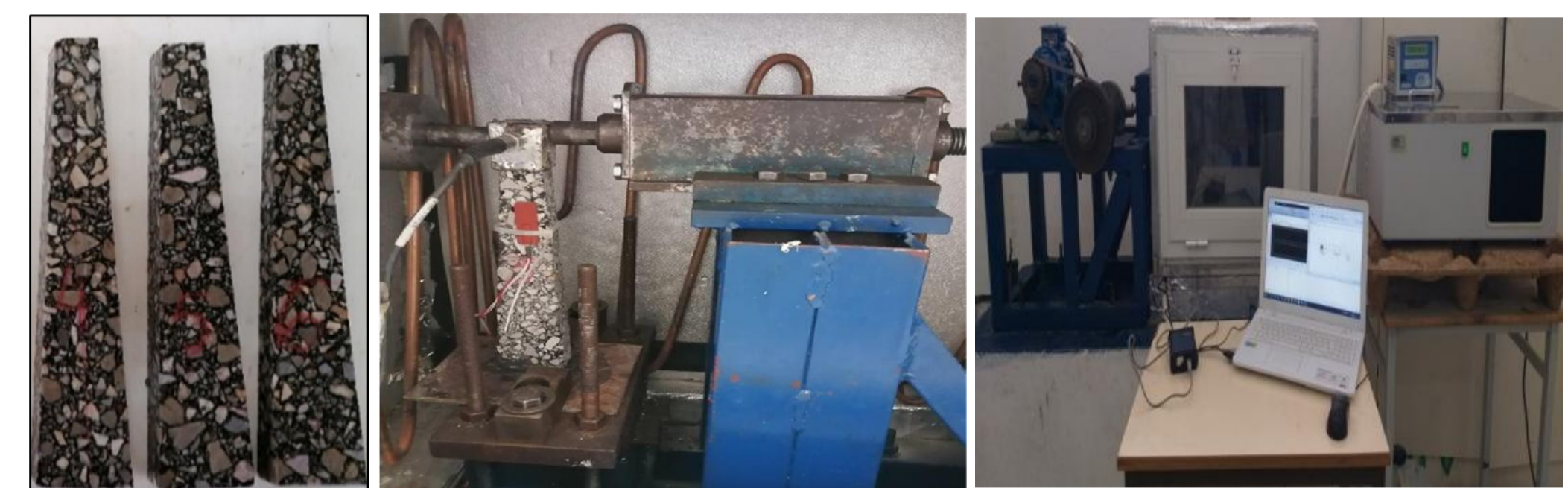
Figure 3. Principe de l'essai flexion 2-points
