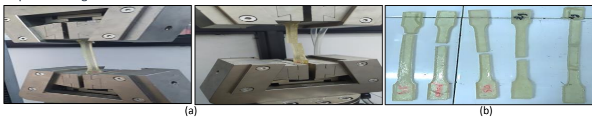
Figure 3: (a) tensile testing instrument and (b) specimens after rupture
