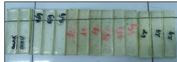
Figure 2: Bending test specimen before fracture
